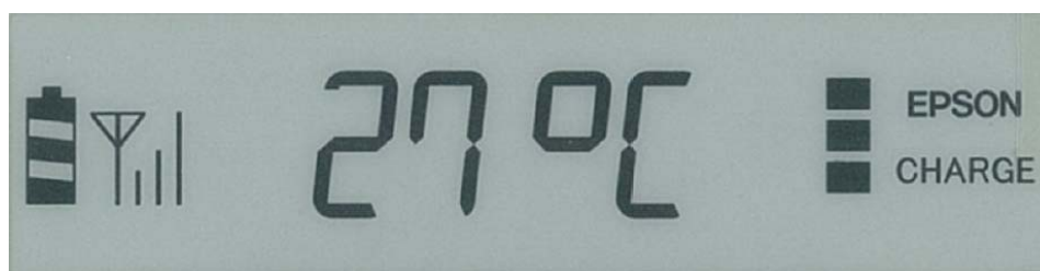
Figure 5.2 Display example of temperature measurement
