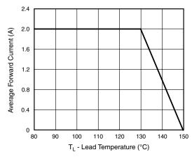
Figure 1. Forward Current Derating Curve
