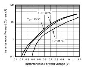
Figure 3. Typical Instantaneous Forward Characteristics
