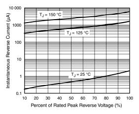
Figure 4. Typical Reverse Leakage Characteristics
