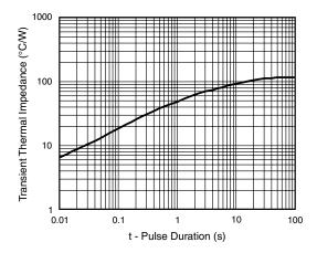
Figure 6. Typical Transient Thermal impedance
