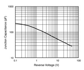
Figure 5. Typical Junction Capacitance
