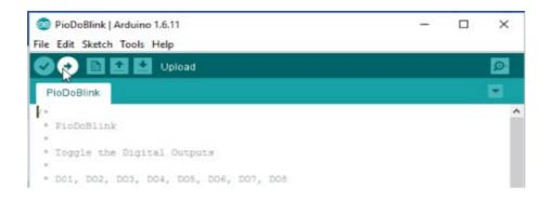
h. After a few seconds the message **'Done Uploading'** is displayed and you can see the LEDs on the board flashing driven by the digital outputs.
