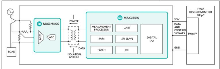
Figure 1. The Sonoma subsystem design block diagram.
