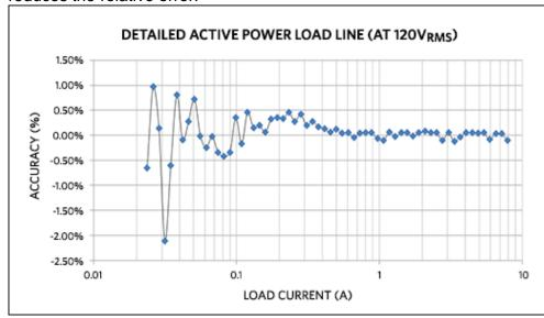
Figure 3. Power accuracy, 23.5mA to 7.9A at 120V<sub>RMS</sub>/60Hz and room temperature.
