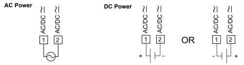
The power supplied to the unit shall employ a 15 Amp UL approved circuit breaker for AC input and a 1 Amp, 250 V UL approved fuse for DC input. It shall be easily accessible and marked as a disconnecting device to the installed unit. This device is not directly intended for connection to the mains without a reliable means to reduce transient over-voltages to 1500 V.
