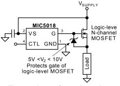
Figure 4. Gate-to-Source Protection
