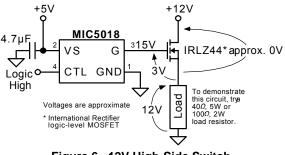
Figure 6. 12V High-Side Switch
