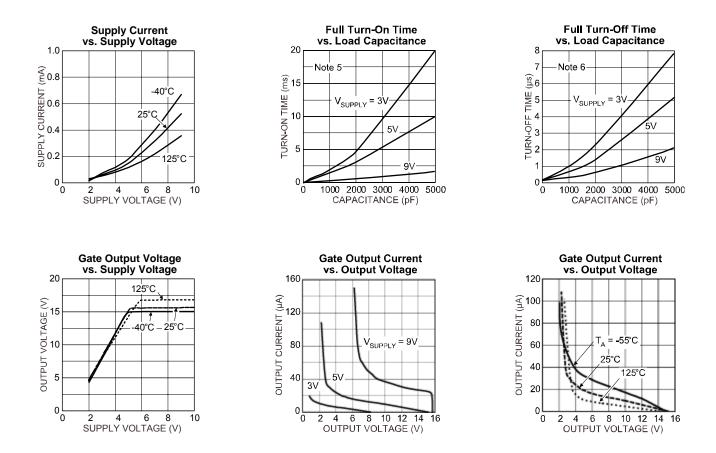
Note 4:  $T_A = 25^{\circ}C$ ,  $V_{SUPPLY} = 5V$  unless noted.
