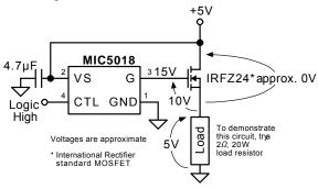
Figure 2. Using a Standard MOSFET
