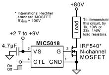
Figure 7. Low-Side Switch Configuration
