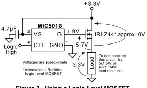
Figure 3. Using a Logic-Level MOSFET
