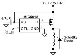
Figure 5. Switching an Inductive Load
